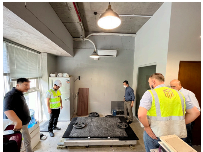
Lien Son Workshop - 120kg Weight drop test on damped spring floating platform
